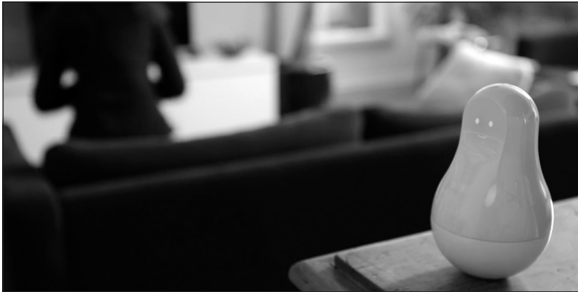
Figure 4.1. The Mother device would collect data from small “motion cookies” attached to household objects. The product, advertised as a “universal monitoring solution,” was briefly available between 2015 and 2018.
